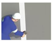
3. Leave it to dry completely for 6 hours. Sand the surface with 150 grit sand paper to achieve a smooth finish.
