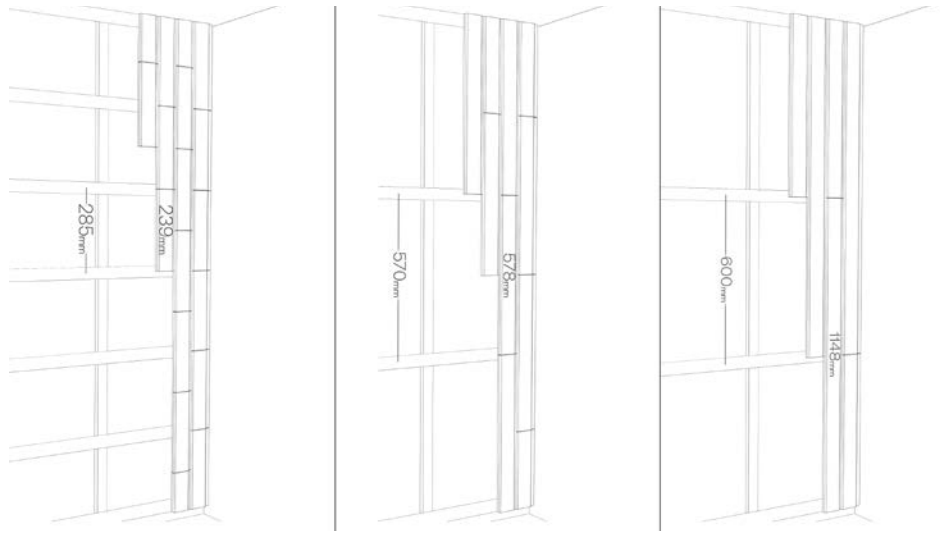
Tiles by Thermory panels vertical installation
