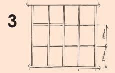
Check framing spacing - 400mm centers for Studs, 800mm nogs and top and bottom nogs to fix ends. Lack of framing will result in a flexible and wavy board surface.
