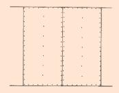
Sheet layout - All edges and board centers must be supported - Sheets to be installed vertically or horizontally. Fixed to nogs & studs for support.
