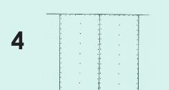
Sheet layout - All edges must be supported - Sheets to be installed vertically. If installed horizontally all free edges must be back blocked
