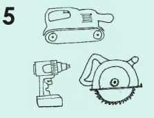
Cutting requires mechanical tools. We recommend using a fine tooth carbide tip saw and clean up with orbital or belt sander.
